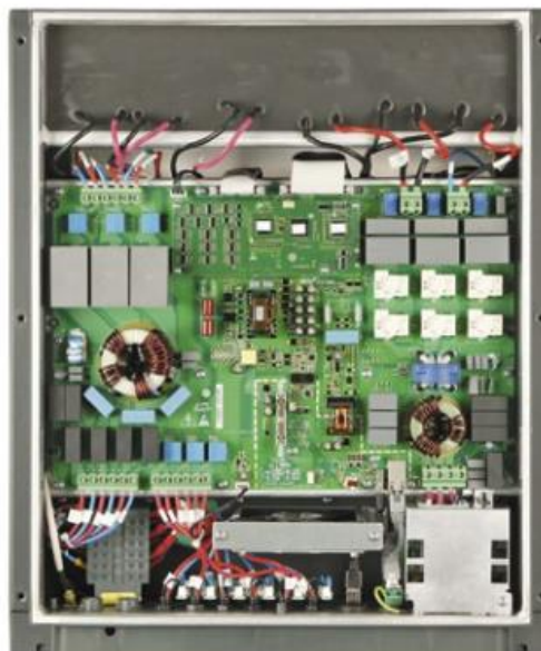
Figure 3-5: SUN2000 Internal Circuits
