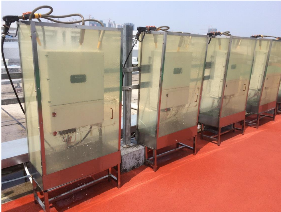
Figure 52. Huawei Inverters Operating in Water Testing
