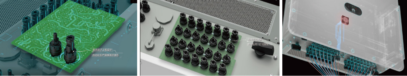
Figure 24 On-board design of Huawei inverter terminals
