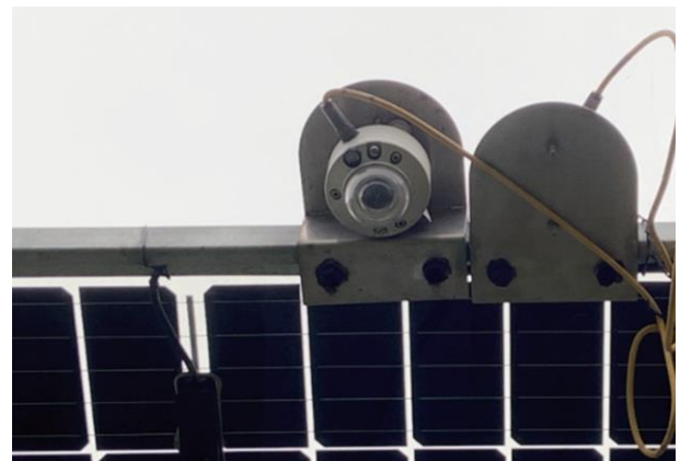
Figure 3-12 Position of the irradiation sensor
