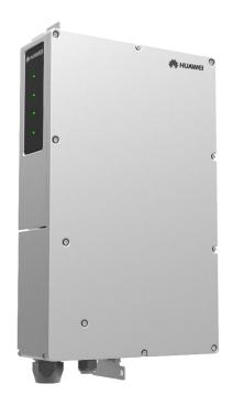
The SmartPID2000 Module is installed in the Smart Array Controller cabinet to reduce the negative effect of the Potential Induced Degradation (PID), and support 1000 V /1100 V / 1500 V DC system.
