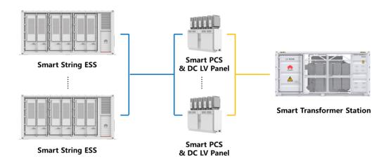
Huawei Smart String Energy Storage System (ESS) Solution involves the Smart String ESS, DC LV Panel, Smart Power Control System (PCS), Smart Array Controller (SACU), Distribution Transformer, and Smart Transformer Station (STS).
