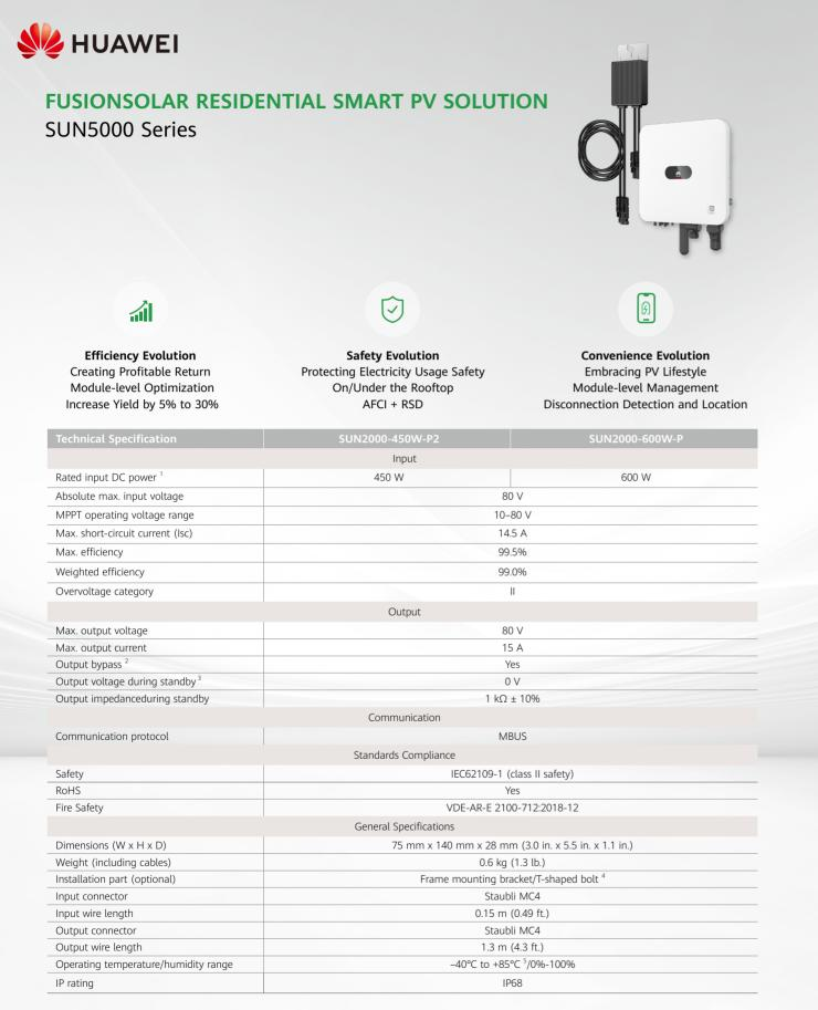
\*1 The maximum power of PV module at STC shall NOT exceed the "Rated Input DC Power" of the power optimizer. PV modules with up to +5% power tolerance are allowed.
