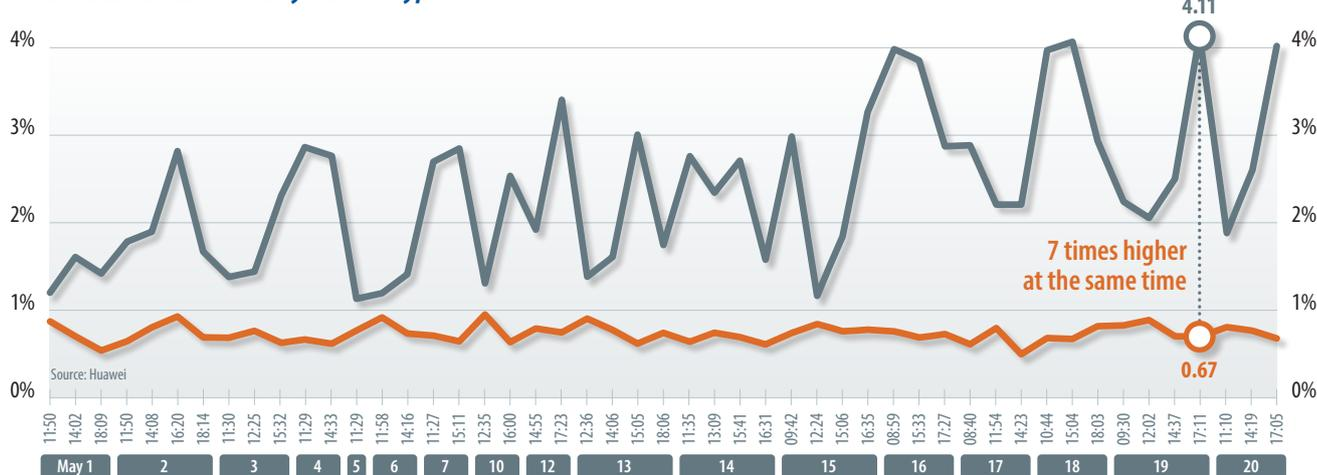
Huawei's inverter THDi is less than **1%**
