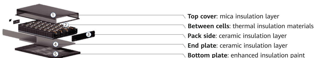
Figure 25 Six-sided insulation for the battery pack
