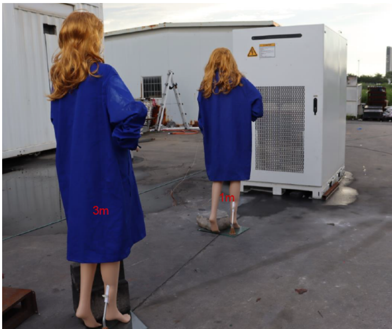
Figure 50 Position of the dummy before the test
