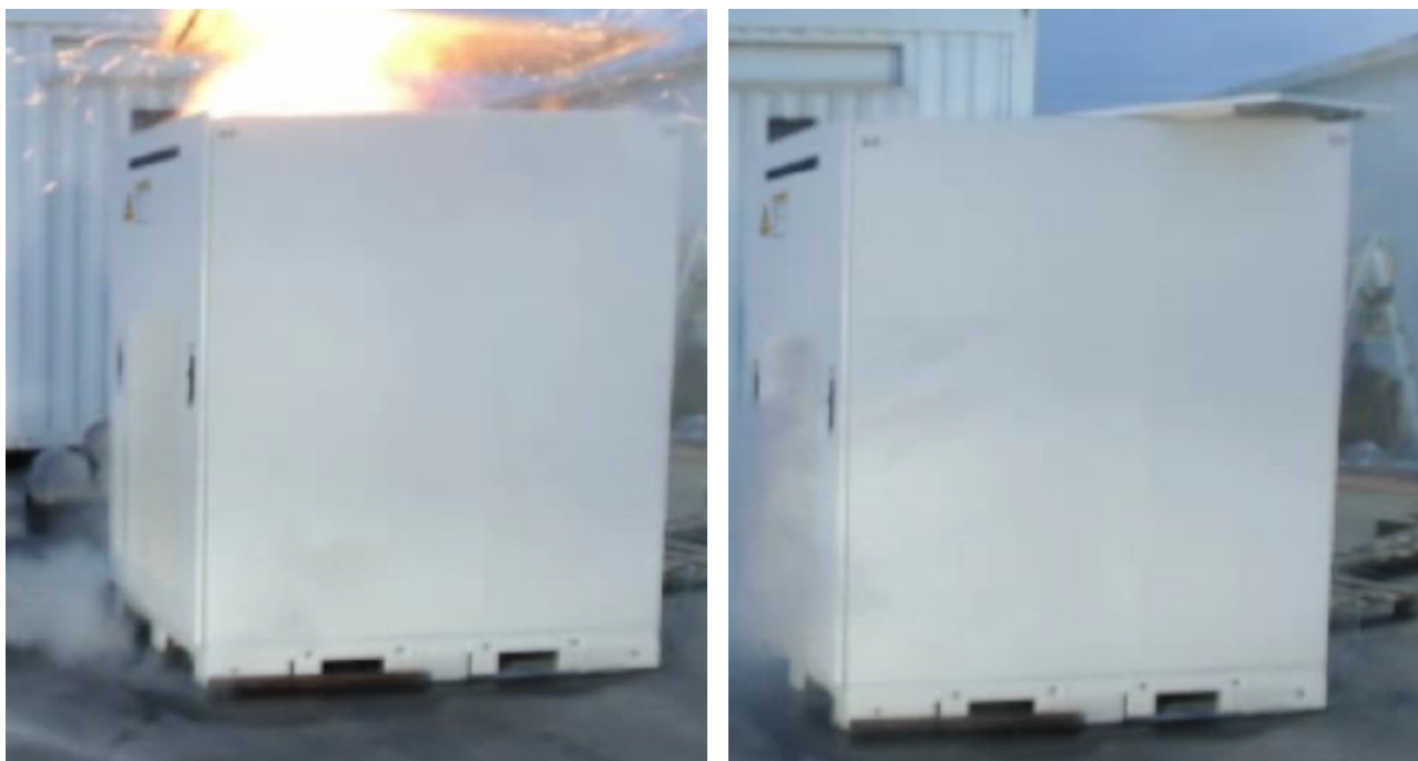
Figure 51 Explosion relief test in progress
