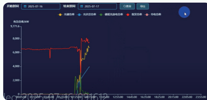
Figure 3-15: Energization/De-energization curves of the 300 kW ball mill in the Mabende mining microgrid project in Congo-Kinshasa
