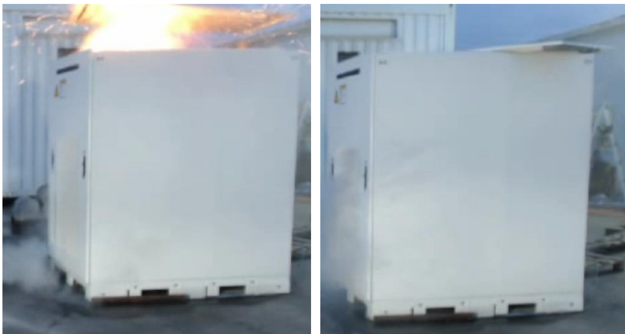
Figure 51 Explosion relief test in progress
