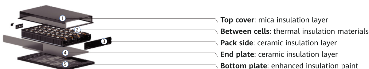
Figure 25 Six-sided insulation for the battery pack
