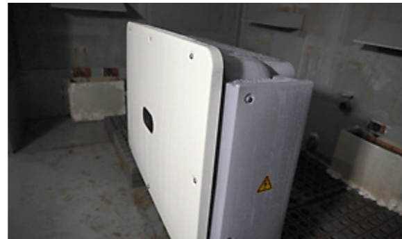
> High-humidity and high-salt spray test
