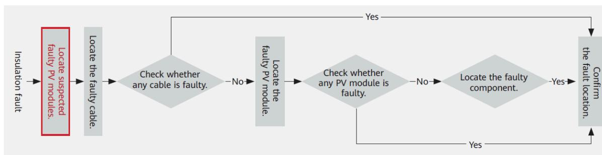
Insulation resistance fault handling process
