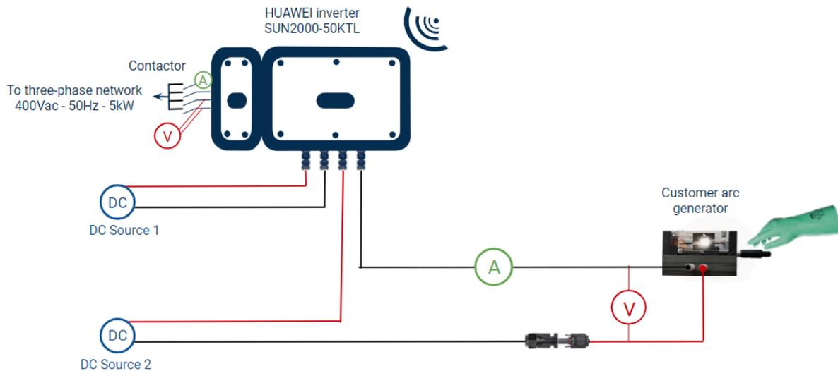
AFCI function test wiring diagram
