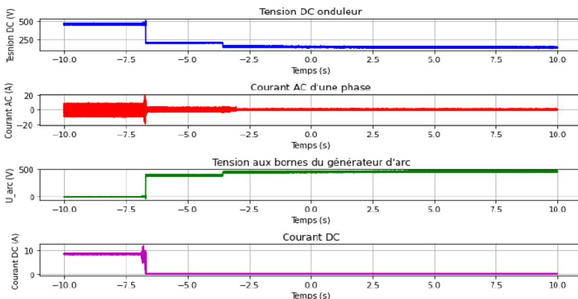
Oscillogram of the AFCI test performed by SuperGrid showing the arc has been detected
