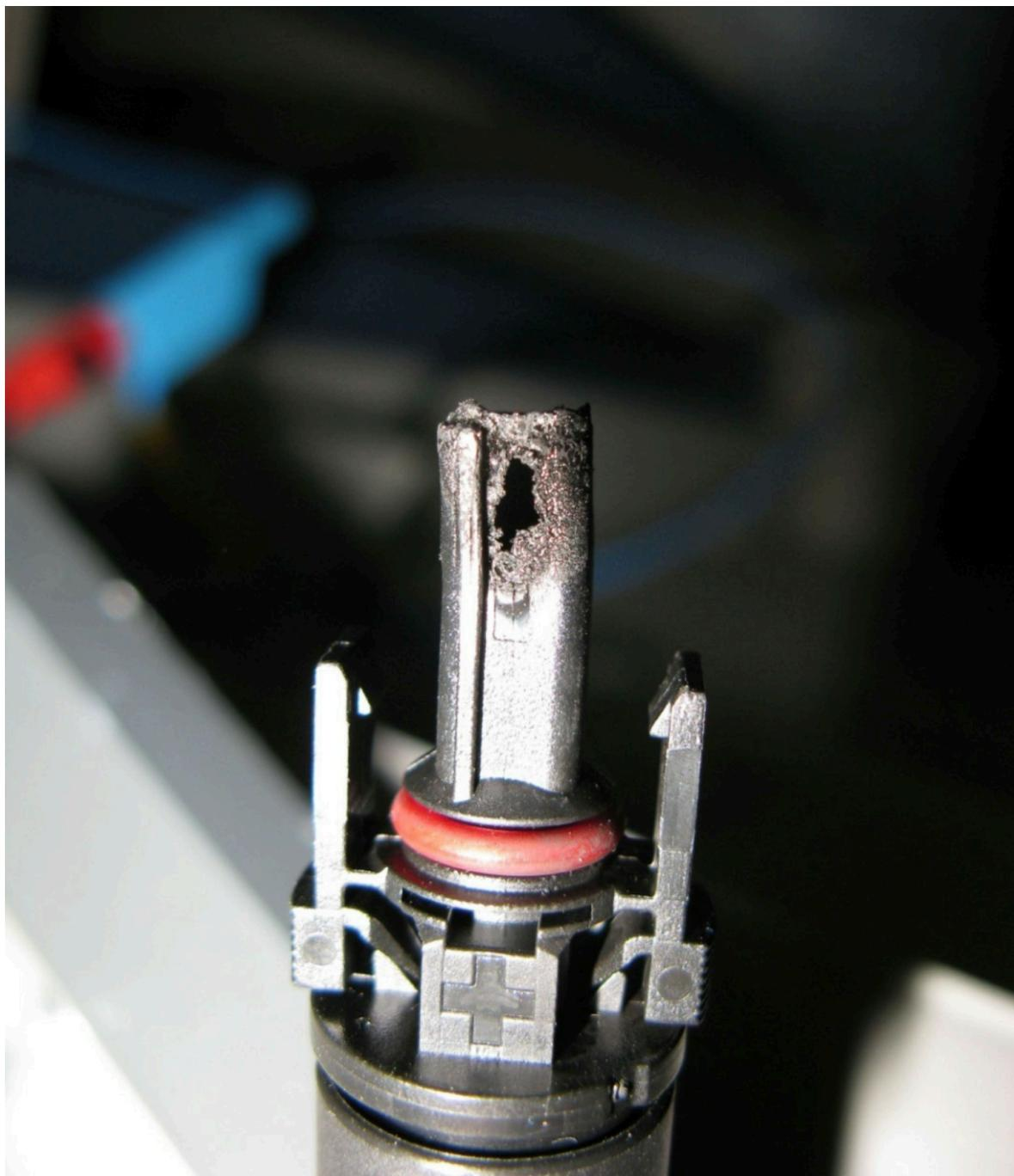
PV module plug connectors damaged by flashing arcs
