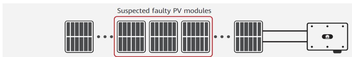
Suspected faulty PV modules located by the Huawei inverter
