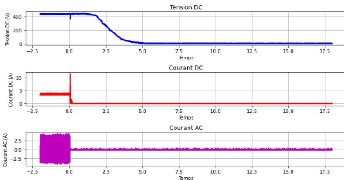
Oscillogram of a Rapid Shutdown (RSD) function test
