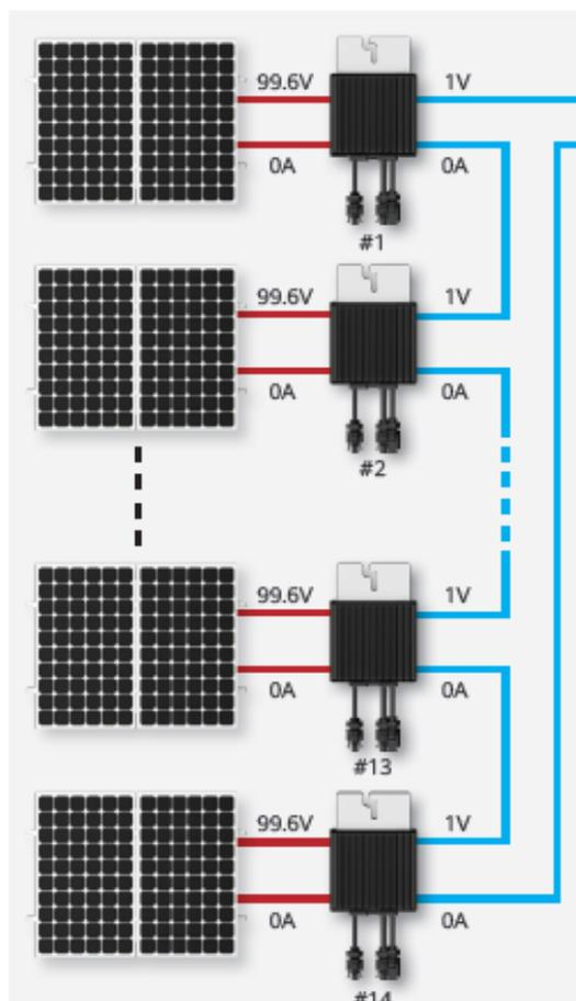
Huawei module-level rapid shutdown solution
