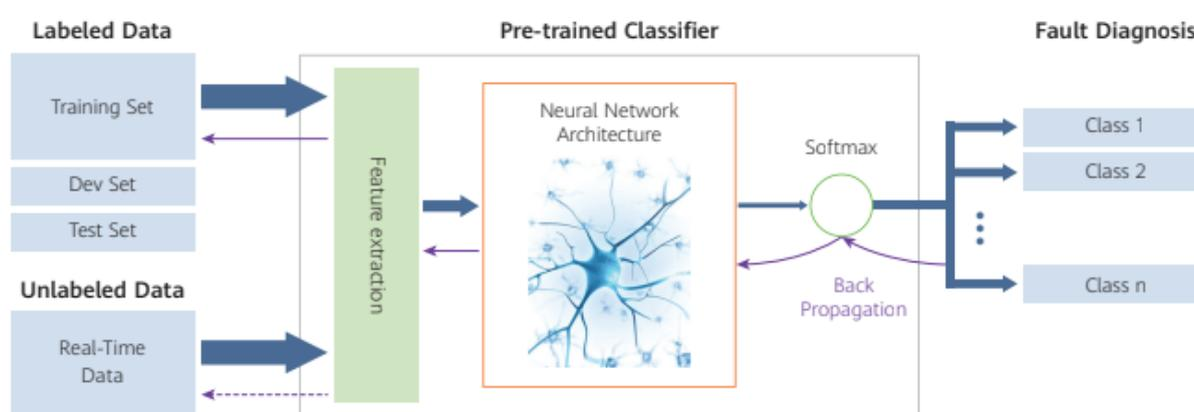
Logical block diagram of the AI solution
