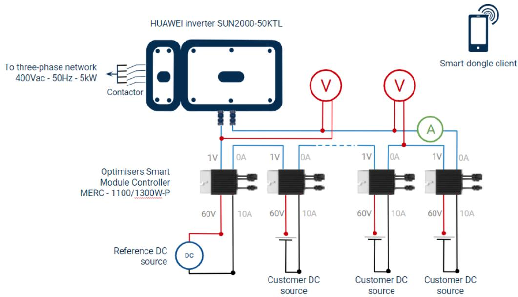
Test diagram for the RSD function
