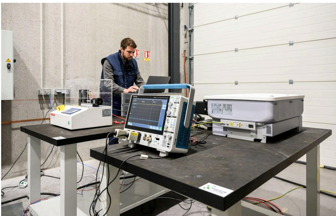
AFCI function test setup in SuperGrid's lab
