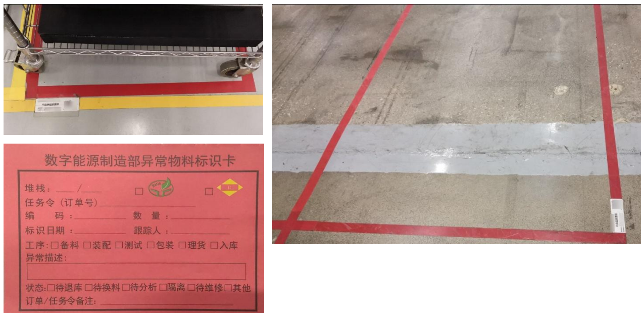
Figure 3-7 Non-conforming inverter PCB and inverter storage area and defective product identification card
