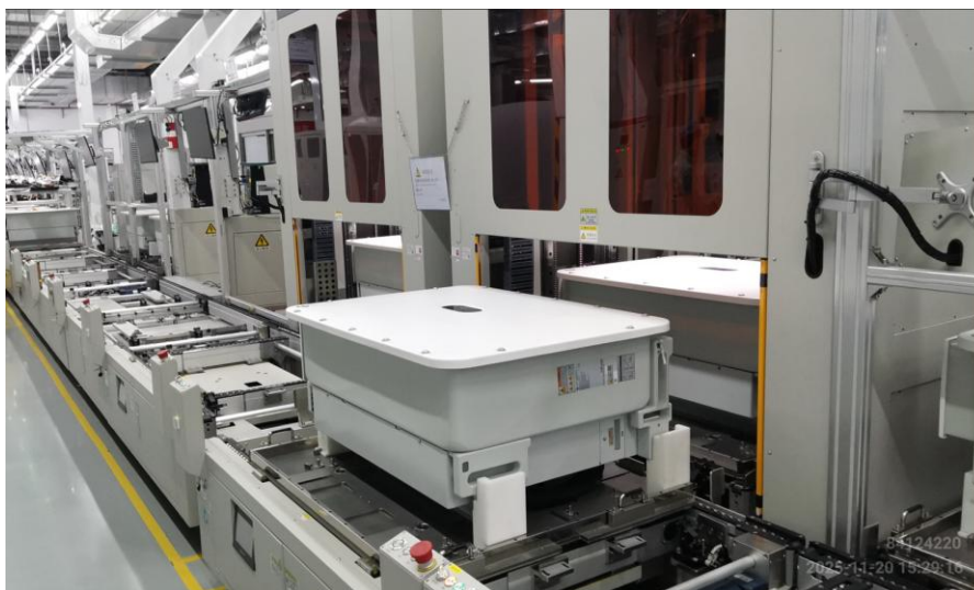
Figure 6-3 Inverter testing in line
