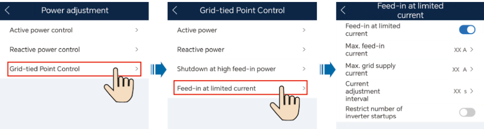
Figure 7-7 Feed-in at limited current
