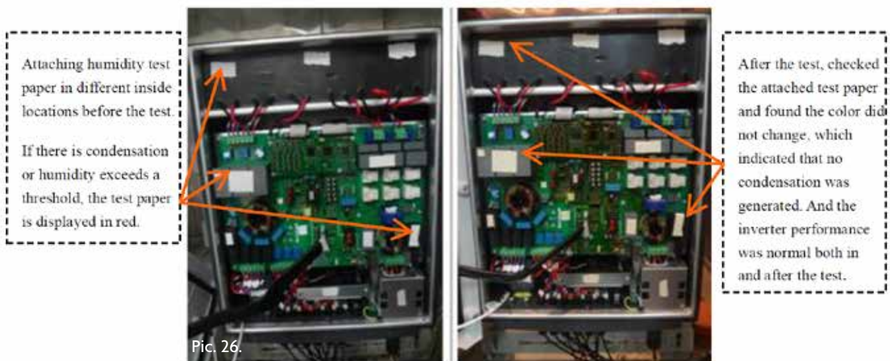
Comparison of Humidity test before and after the rain
