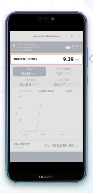
The current power tile shows how much power your system is currently generating. Production typically peaks in the middle of the day when the sun is the most powerful and highest in the sky.
