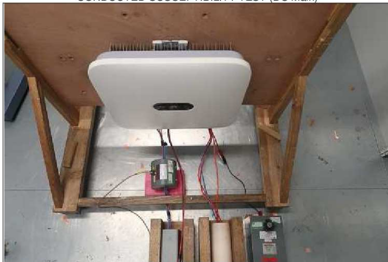
CONDUCTED SUSCEPTIBILITY TEST (DC Main)
