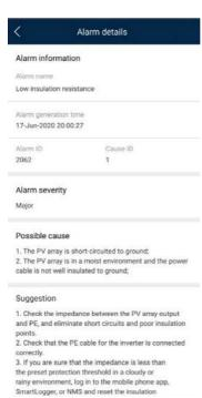
When user monitoring the PV plant registered in FusionSolar App, the low insulation resistance alarm or fault can also be indicated via following interface by:
