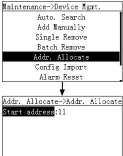
Press enter to confirm the address assignment:
