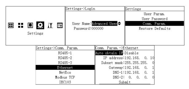
The default IP for Smartlogger1000 is 192.168.0.10 and if your local IP of your router is 192.168.0.1 you can leave the default Ethernet parameters like it is and the Smartlogger1000 will be able to connect with the router.
