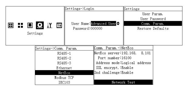
If you have the option Network test you can made a test to see if your Smartlogger1000 is connected to the server. The default port number is: 16100. If this option is not available then call the service team to check if your Smartlogger1000 is connected to the server and ask them to create the PV plant and account for you.
