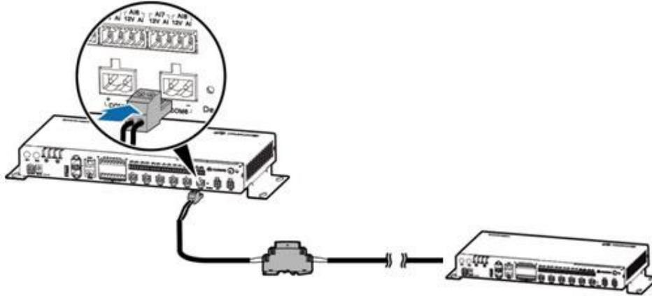
Set the RS485-3 port to the slave mode on the web client. Log in as to the embedded WebUI as an advanced user, click the **Settings** tab, and choose **Comm. Param.** > **RS485**. Set **Protocol** to **Modbus-Slave** for RS485-6, and click **Submit** to enable the slave mode.
