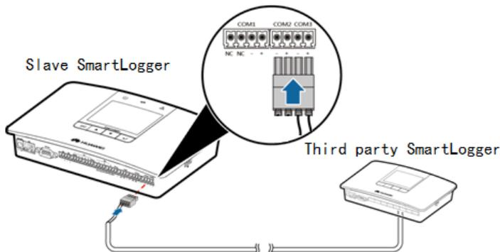
Set the RS485-3 port to the slave mode on the web client.
