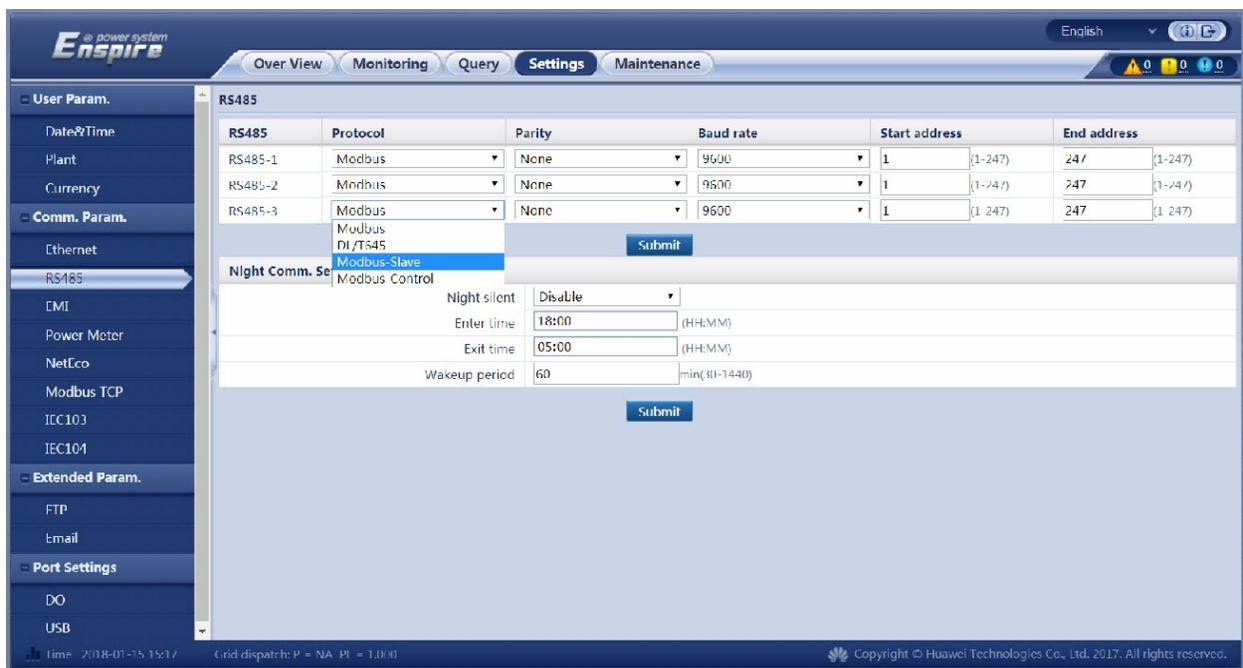
After the slave mode takes effect, connect the devices including inverters to COM1 and COM2.
