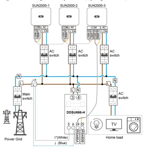
Balanced three-phase grid connection
