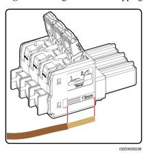
$Step\ 2\quad \hbox{Connect the AC connector to the AC output port.}$
