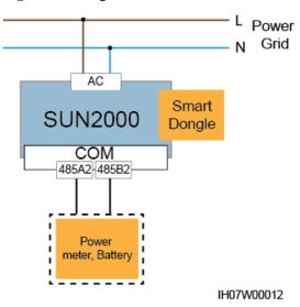
Figure 5-20 Connecting cables to the power meter (single SUN2000)
