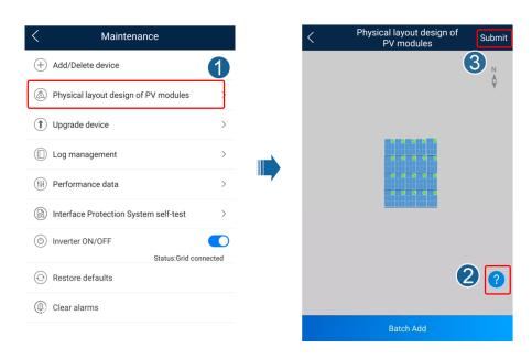
**Step 2** Set the physical layout of smart PV optimizers on the WebUI of the FusionSolar Smart PV Management System (https://intl.fusionsolar.huawei.com).
