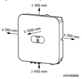
When installing multiple SUN2000s, install them in horizontal mode if sufficient space is available and install them in triangle mode if no sufficient space is available. Stacked installation is not recommended.
