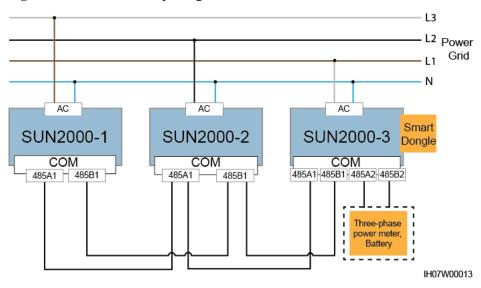
Figure 5-23 Balanced three-phase grid connection
