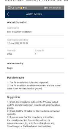
• When user monitoring the PV plant registered in FusionSolar App, the low insulation resistance alarm or fault can also be indicated via following interface by :
