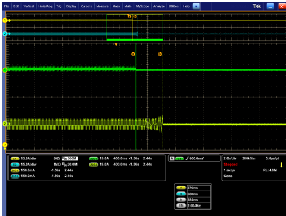
Disconnection at P_{AC} 0% and Q_{AC} 0% reactive load and 33% nominal power
