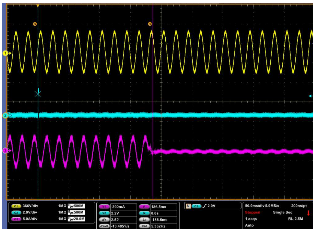
Diagram of under-voltage protection:L2 phase
