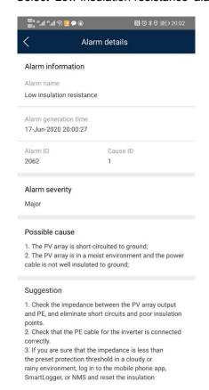
When user monitoring the PV plant registered in FusionSolar App, the low insulation resistance alarm or fault can also be indicated via following interface by:
